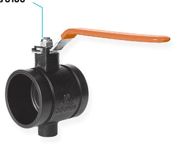
The Series 8100 Low Profile Butterfly Valve has a rated working pressure of 300 psi (20.7 bar) and provides efficient control of fluid in piping systems. Flow can be from either direction and the valve may be positioned in any orientation. The ductile iron body is epoxy-coated to resist atmospheric corrosion. The disc is EPDM encapsulated ductile iron compatible with a variety of chemicals and temperature ranges.
